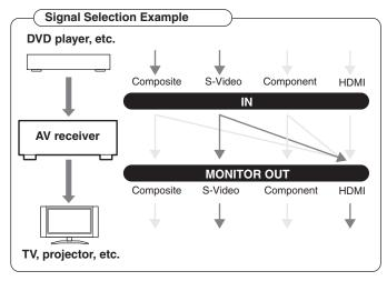
The onscreen setup menus appear only on a TV that is connected to the HDMI OUT. If your TV is connected to the composite video or S-Video MONITOR OUT, or the COMPONENT VIDEO OUT, use the HT-R667's own display when changing settings.
